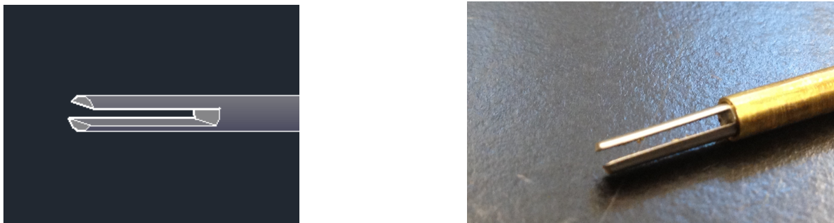
Figure 1. Stainless Steel Rod with 1mm slot 10-15mm deep for sample to mount in slot (left). Steel fork and Copper tubing (right).
