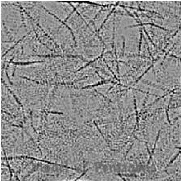
FIG. 5: Strong phase-object simulation of 0.19 nm resolution HREM image from a collection of randomly-oriented atom-thick hexagonal graphene flakes with a cyclopentane at their center.
