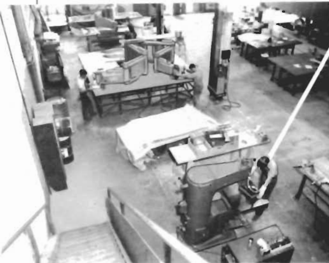
RADIAL ARM ROUTERS —Through use of high speed spindles in routing and drilling, accuracy can be improved at economical costs.
