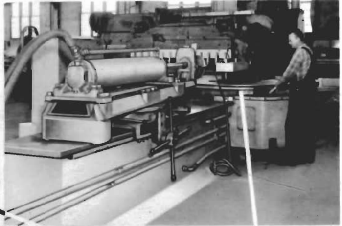
CONTOUR FORMING —Through use of this equipment complex sheet metal parts and extruded shapes may be formed.
