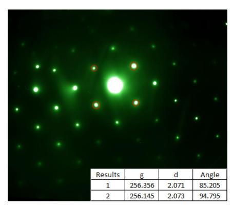
Typical SAED diffraction data obtained from a possible ZrC inclusion in  $ZrB_2$  ceramic. The inset table shows the results of our 4spots plugin run using the points circled in red. The indicated results rule out the possibility of ZrC, but suggest the presence of an unexpected phase  $B_4C$ .
