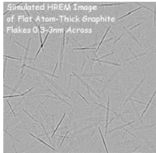
FIG. 2.—Strong phase-object simulation of 0.19 nm resolution HREM image from a collection of randomly oriented atom-thick hexagonal graphene flakes.
