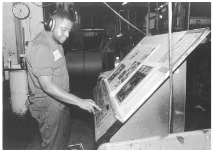
Printing machine operators prepare, operate, and maintain the printing presses in a pressroom.
