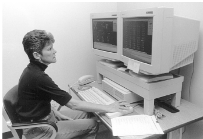
Power plant operators often use computers to keep records of switching operations and loads on generators, lines, and transformers.
