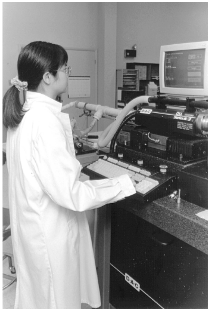
A contact lens manufacturing worker grinds lenses according to prescription.
