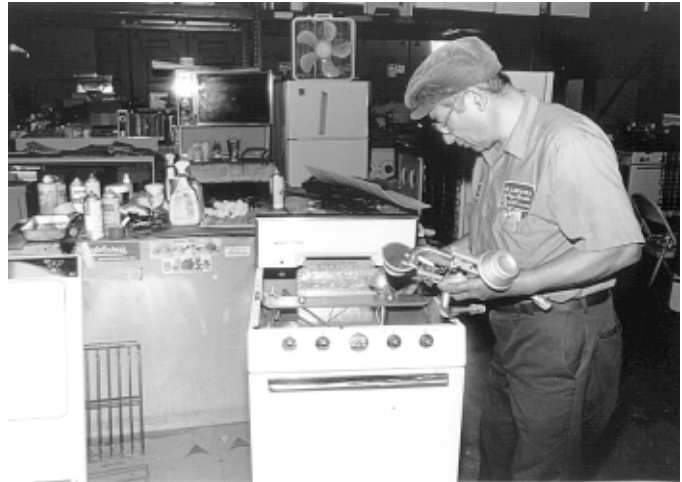
Gas appliance repairers check the heating units of stoves and may replace defective parts.
