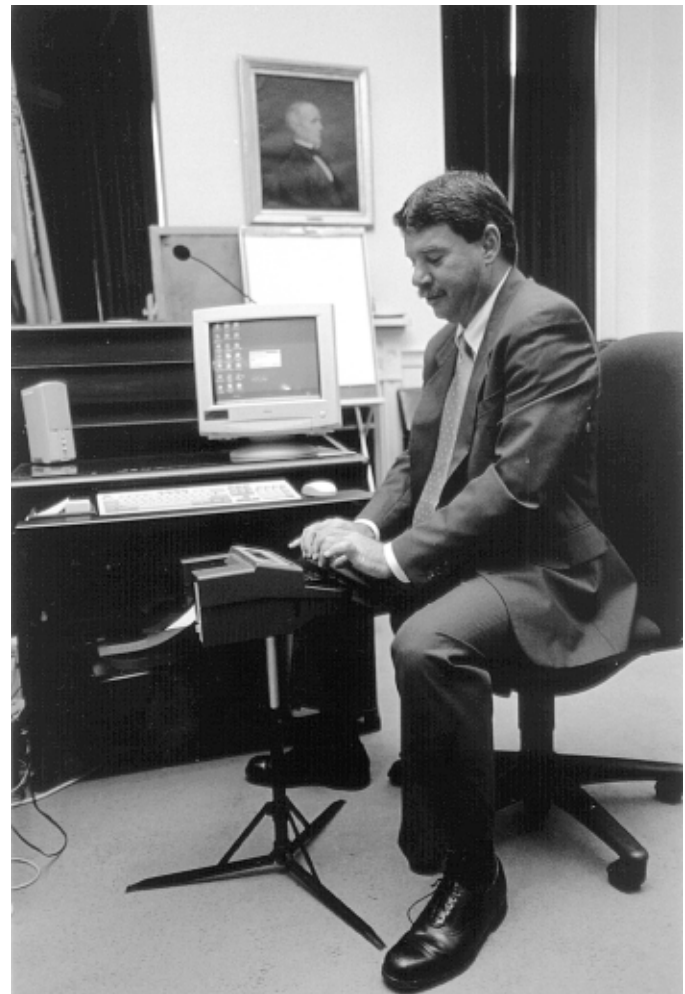
Court reporters use stenotype machines to take verbatim reports of speeches, conversations, legal proceedings, meetings, and other events.
