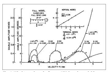
Fig. 1. Wind-tunnel results from a 1/50th-scale model Tacoma Narrows Bridge.<sup>3</sup> The wind velocity in the wind tunnel of 5 ft/s (1.5 m/s) is equivalent to a wind velocity of 35 mph (16 m/s) for a full-size bridge.
