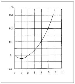
Fig. 3. The values of  $A_2$  as a function of wind velocity, U, from wind tunnel measurements.<sup>4</sup> A U of 5 is approximately equivalent to a wind velocity of 27 mph (12 m/s) for a full-size bridge.
